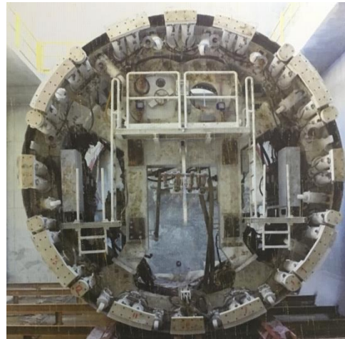
Figure 8. A picture of the shield machine that workers used to dig out the tunnel.
