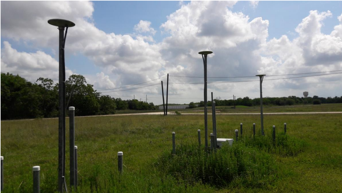
Three extensometers at the UH Coastal Center
